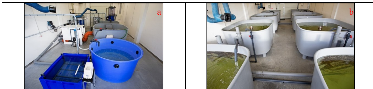
Figure 15: Pilot case for recirculating aquaculture system for shrimp cultivation in Klaipėda University Business Incubator: water preparation and filtration system (a) and shrimp growing tanks (b).
